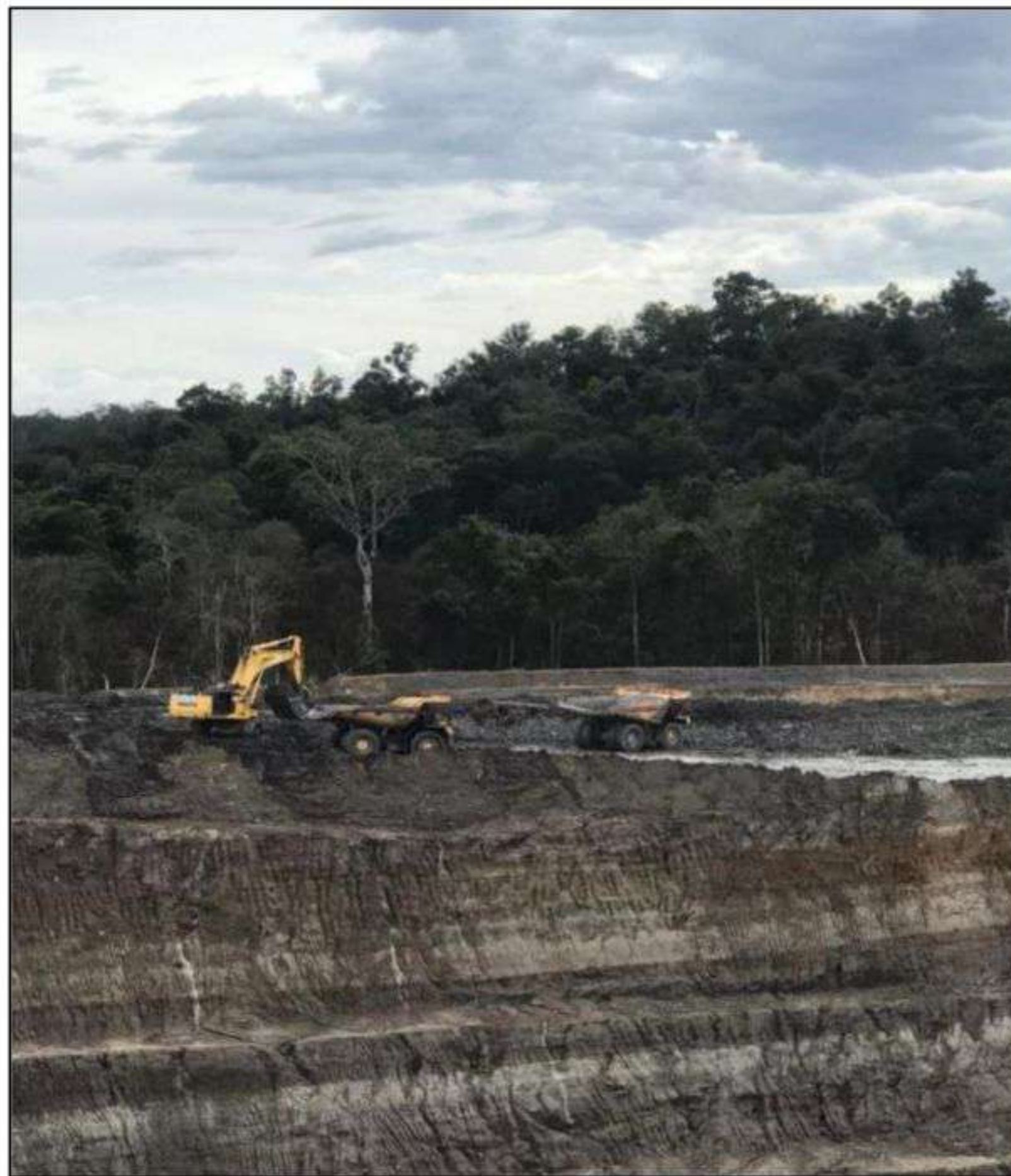
Gambar 4.2 Metode Top loading
