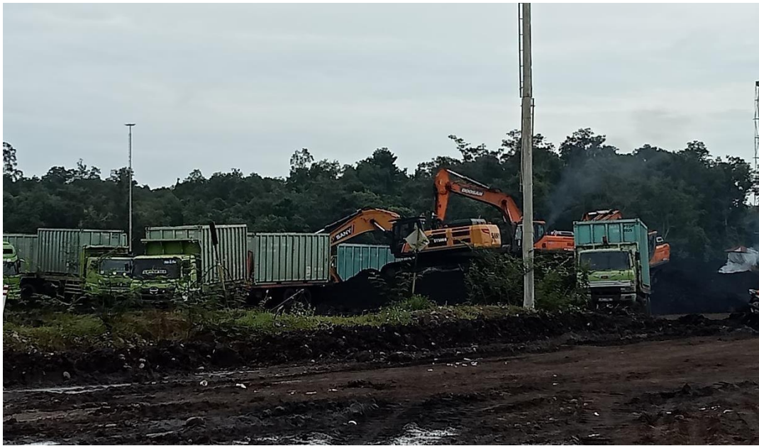
Gambar A.1. Proses loading batubara ke Dump truck
