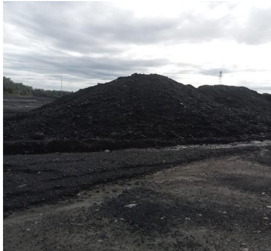
Gambar 4.2 Pola Penimbunan Kerucut ( Conical Stack )
