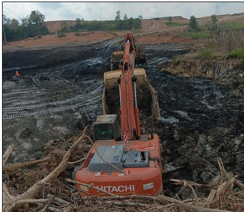
Gambar 2.12 Kegiatan Coal Cleaning
